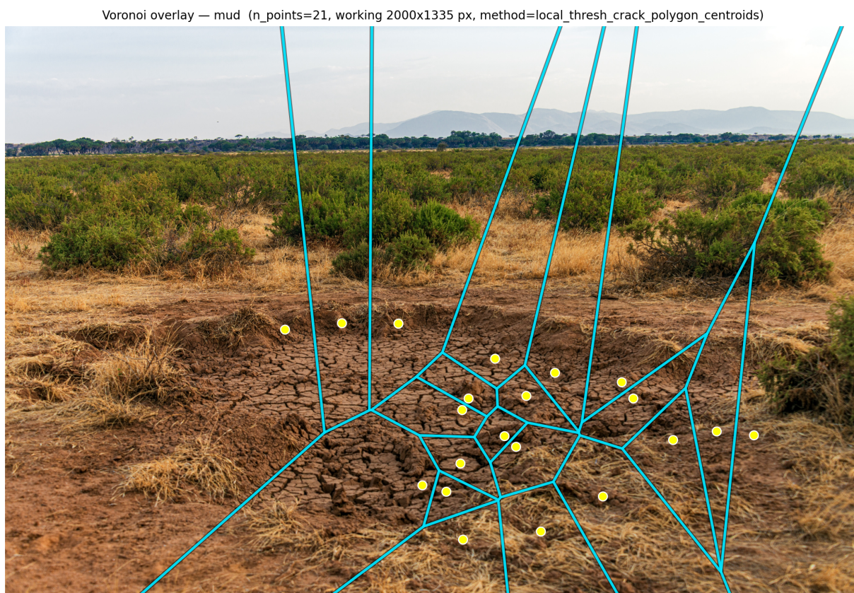
Figure 4: Voronoi overlay on a dried-out elephant mudwallow in Samburu National Reserve, Kenya (Wikimedia Commons, CC-BY-SA 4.0). Cyan dots: centroids of the polygonal mud islands ( n = 21 ), extracted by local thresholding on the brown mud ROI. Cyan lines: the Voronoi tessellation on those centroids.
